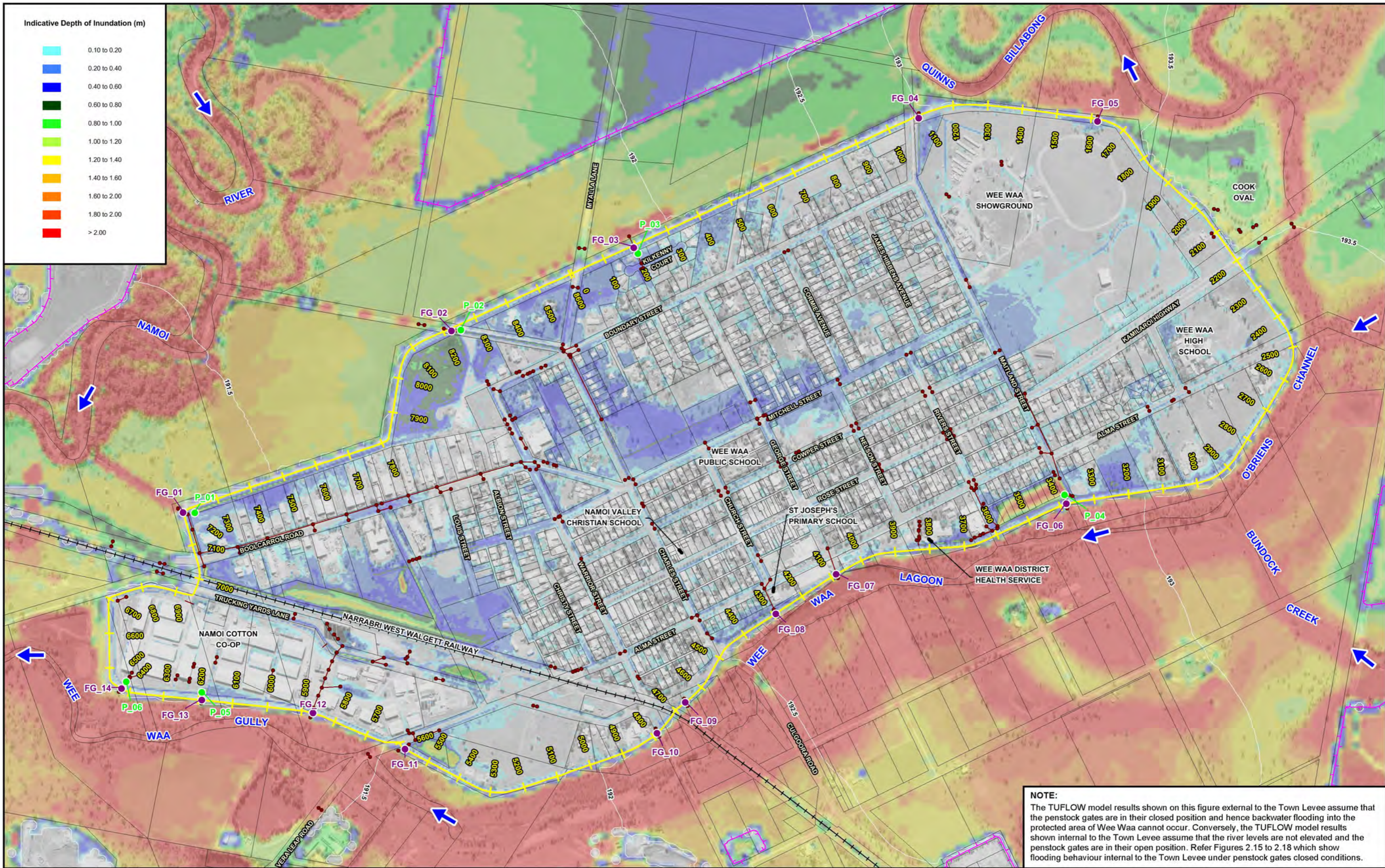
Figure 2.5 (Sheet 2 of 2) INDICATIVE EXTENT AND DEPTHS OF INUNDATION 1% AEP
