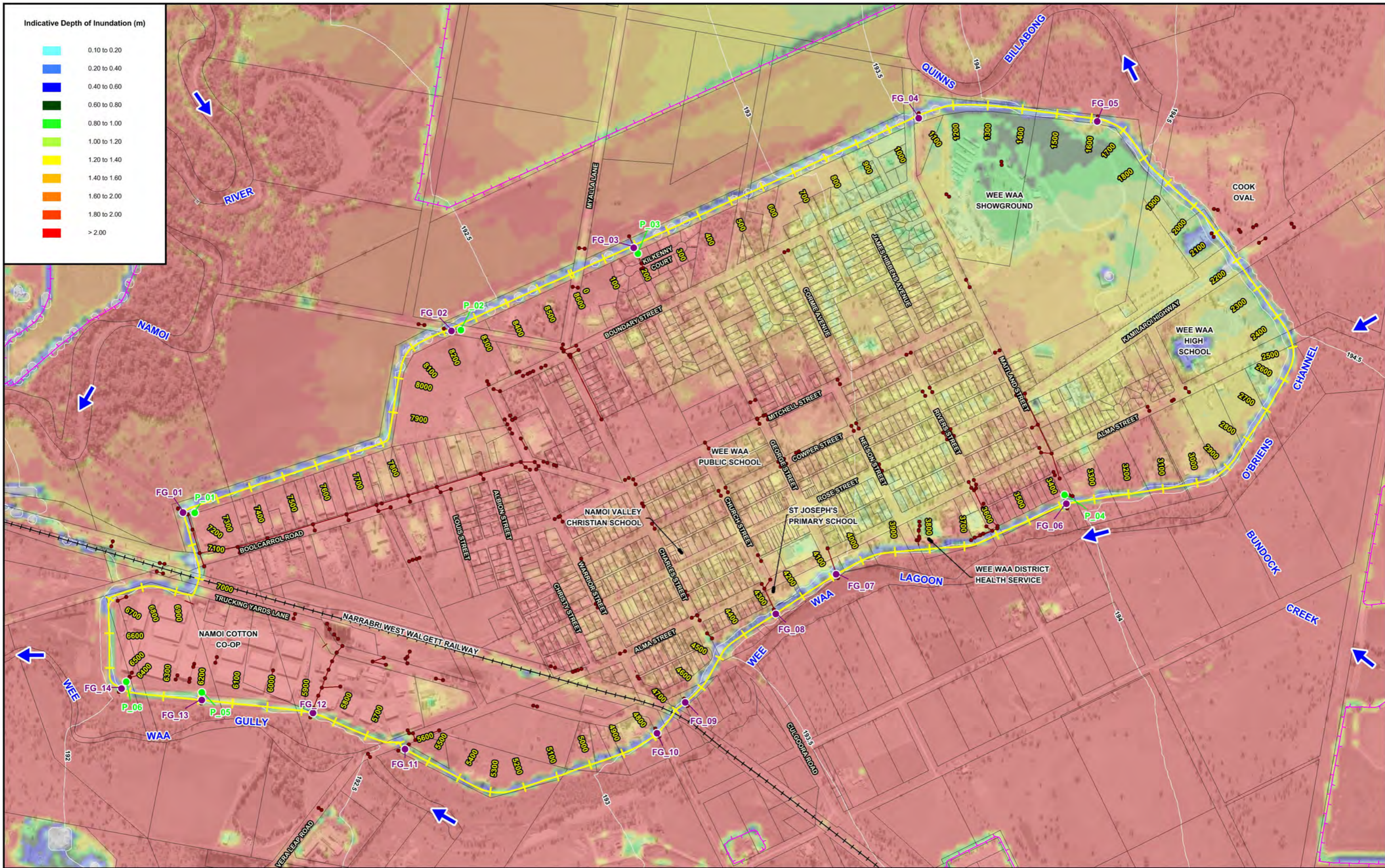
Figure 2.8 (Sheet 2 of 2) INDICATIVE EXTENT AND DEPTHS OF INUNDATION EXTREME FLOOD
